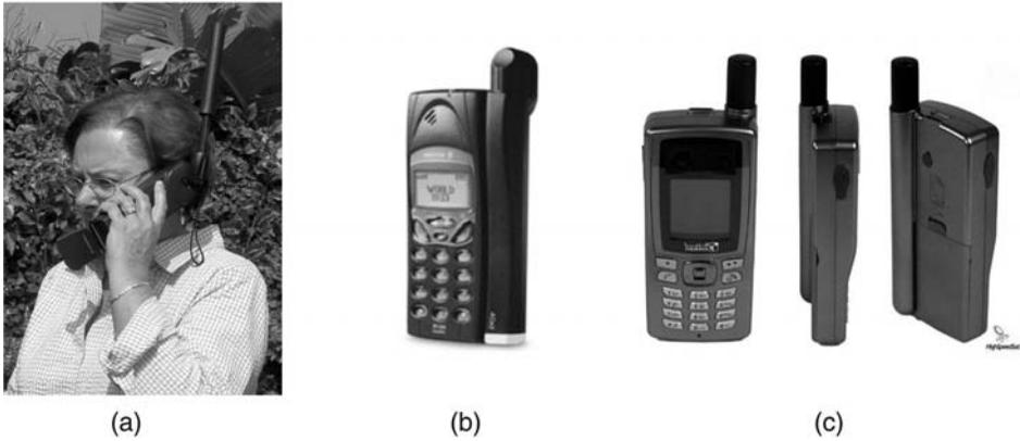
**Figure 9.37** A selection of hand-held MSS satellite phones; the Iridium phone is shown fully deployed while the Inmarsat and Thuraya phones are collapsed in their storable configurations. (a) Iridium (Motorola) 9500, (b) Inmarsat iSatPhone, and (c) Thuraya SO-2501 ([www.highspeedsat.com](http://www.highspeedsat.com)).
