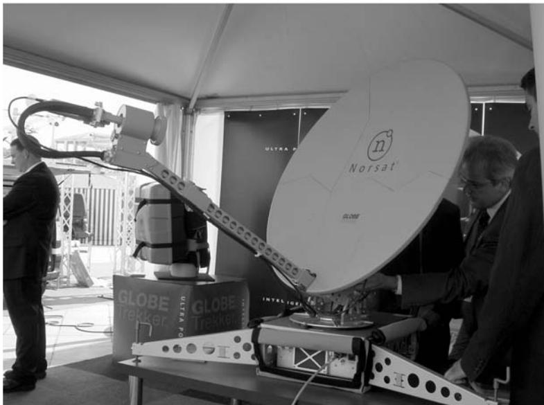
**Figure 1.9** Highly transportable Ku-band Earth station for disaster recovery and temporary applications.
