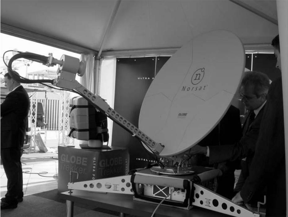
**Figure 9.5** Portable Ku-band Earth station for two-way broadband services; this terminal is capable of automatically acquiring a satellite once set up.
