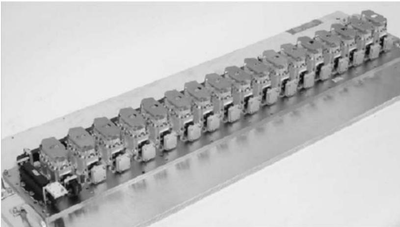
**Figure 6.29** Temperature compensated Ku-band output multiplexer. (Courtesy of COMDEV International.)
