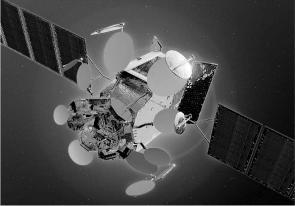
**Figure 7.7** The Astrolink satellite design incorporated eight reflector systems, each with up to eight individual feedhorns to produce a like number of spot beams [1].
