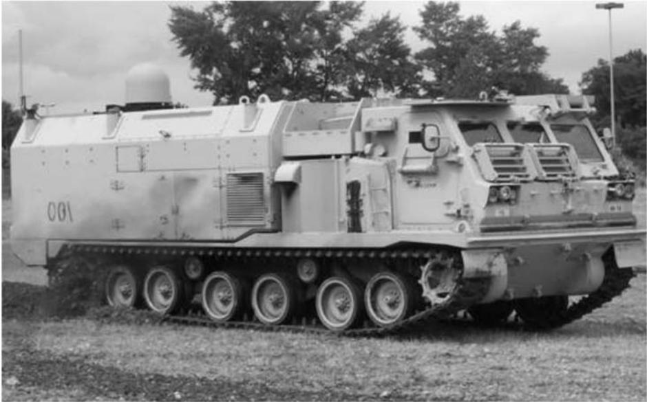
**Figure 9.7** Ku-band Earth station mounted on a military troop carrier capable of communications on the move. (Courtesy of Datron L-3 Communications.)
