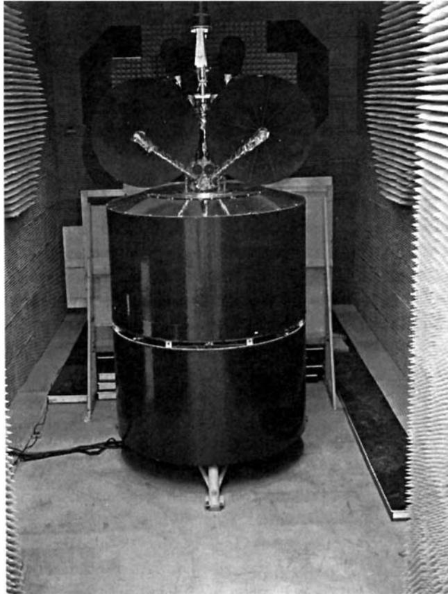
**Figure 2.4** The Intelsat IV spacecraft. (Source: Photograph courtesy of Hughes Aircraft Company.)
